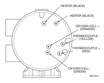
Figure 4-6. Termination Housing Connections
